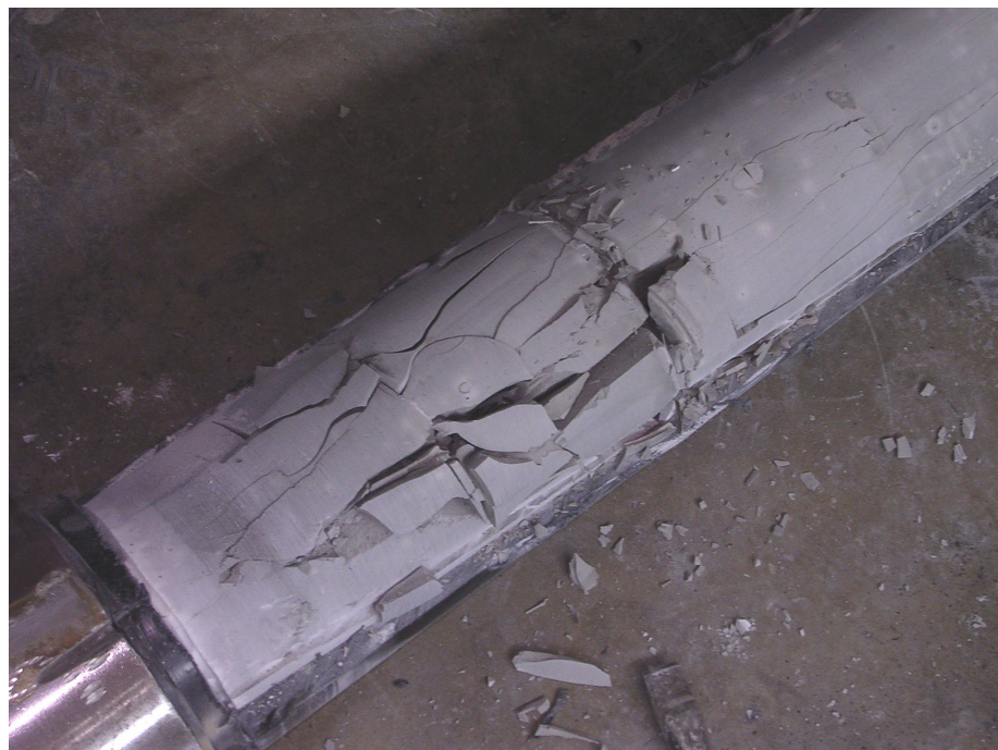
Figure 4-88: Grout at tower end immediately after opening - Specimen 10
