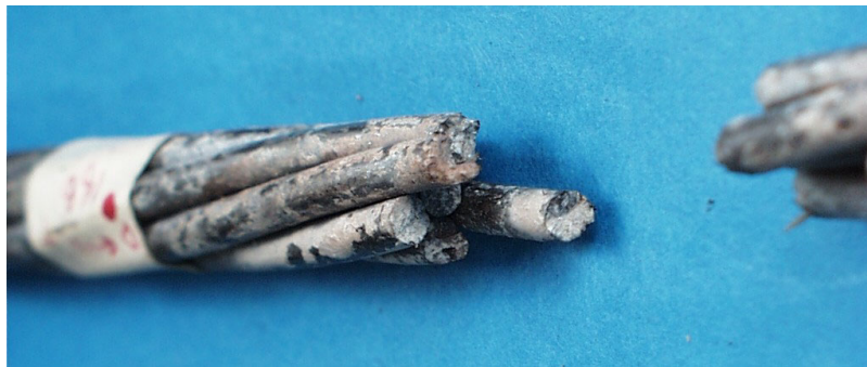
Figure 4-39: White substance on strand 17 at midspan - Specimen 7
