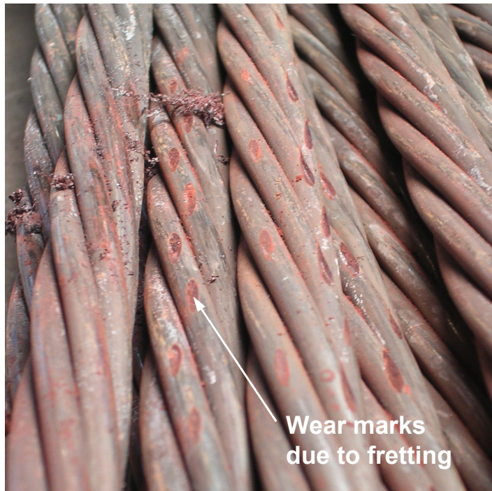
Figure 4-56: Wearing of the strands due to fretting - Specimen 8
