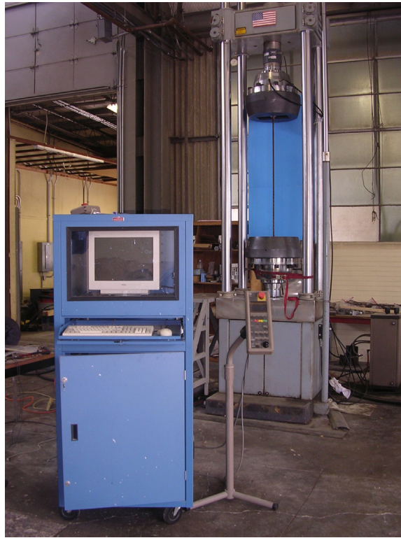
Figure 3-1: 220-kip MTS load frame
