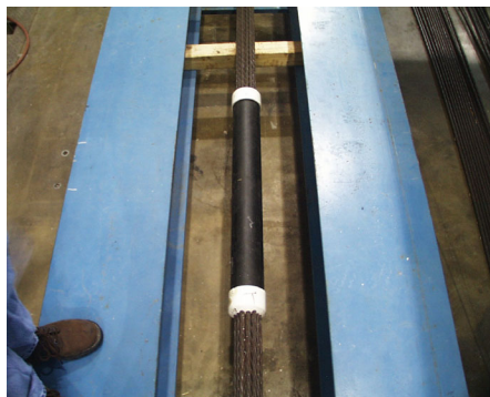
(a) Grouted section in clamp region (b) PVC end cap sealed with caulk
