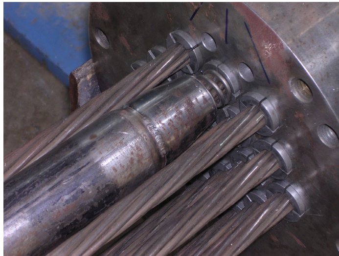
Figure 2-14: Tapered adapter used for mono-strand stressing
