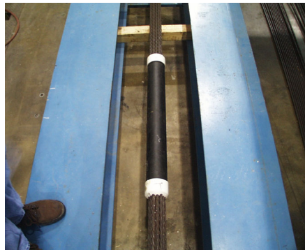
Figure 2-11: PE pipe and white PVC end caps used on ungrouted specimens
