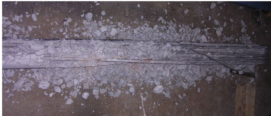
Figure 4-73: Grout condition under the load point - Specimen 9
