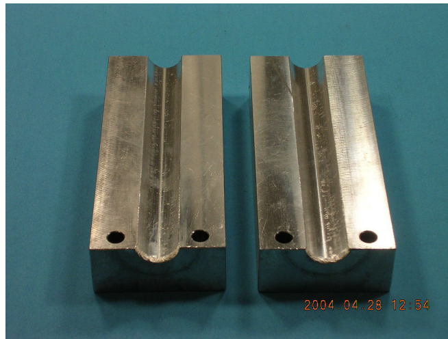
Figure 3-4: New aluminum grips used for axial fatigue testing
