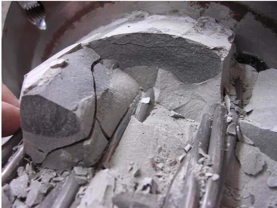
Figure 4-72: Grout void at tower anchorage - Specimen 9
