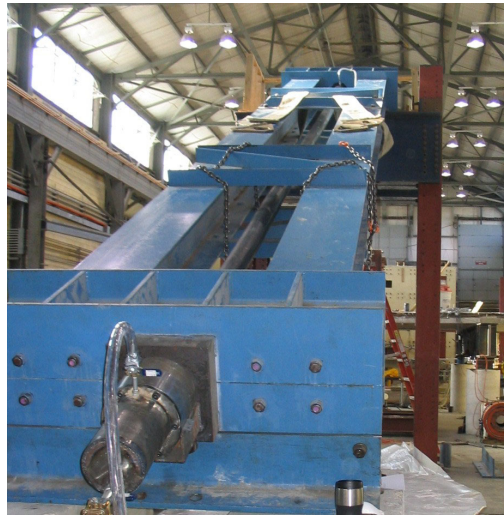
Figure 2-17: Inclination of stay for grouting
