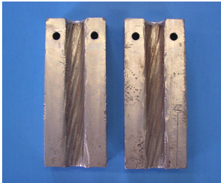
Figure 3-6: Grips after use in multiple axial fatigue tests
